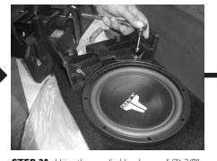
**STEP 20:** Using the supplied hardware of (2) 3/8"- $16 \times 1$ " hex bolts, (2) 3/8" flat washers and (2) lock washers. Attach this drilled out position of the black console, to the rear of the enclosure.
